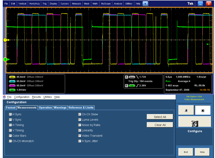
Measurement Selection Menu (Option VGA).
