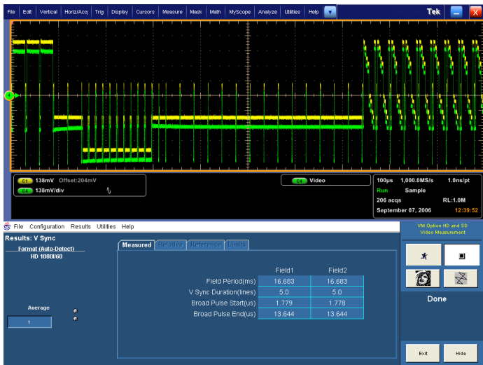
V Sync Display (Option SD and HD).
