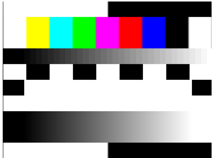
PC Graphics Matrix Test Signal (Option VGA).
