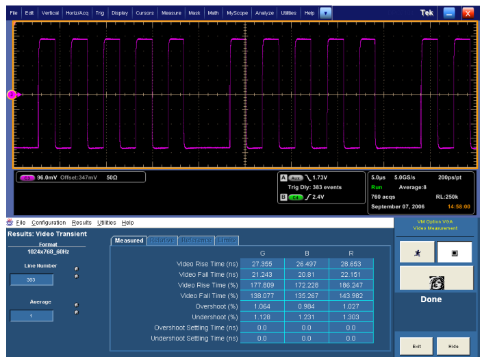
RGB Transient Response Measurement Results (Option VGA).
