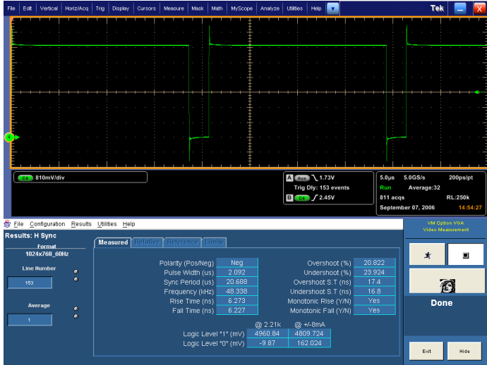
H Sync Measurement Results (Option VGA)
